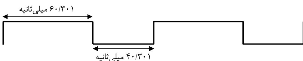
$$f = \frac{1}{T1 + T2} = \frac{1}{60.301 \text{ ms} + 40.301 \text{ ms}} = 9.94 \text{ Hz}$$
